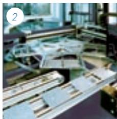
2. Automatic loading station of an in-line PE-CVD deposition system for anti reflective and passivation coatings on c-Si solar cells
