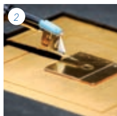
2. Experimental characterisation of a concentrator solar cell ©FRAUNHOFERISE
